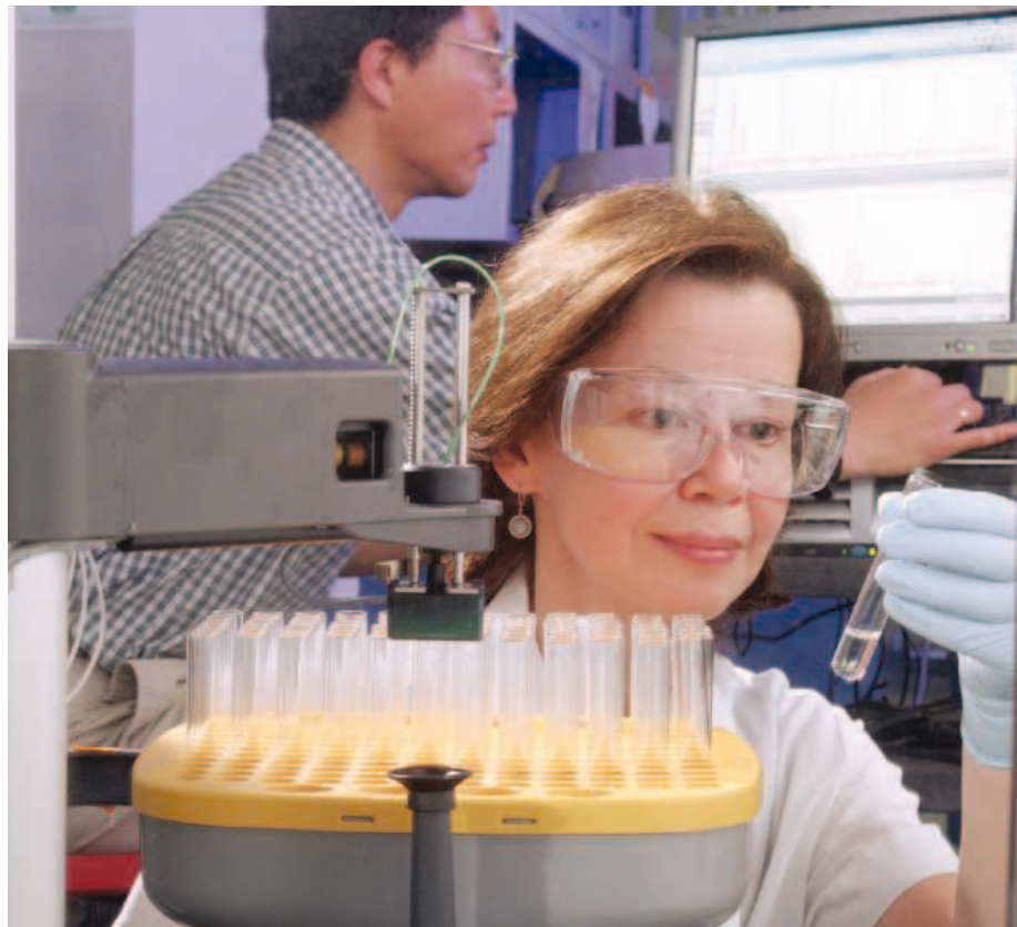
Pure speed. Researchers at the Midwest Center for Structural Genomics use robotic gear to speed protein purification.
